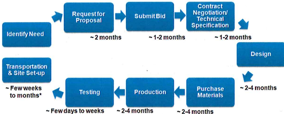
Figure 4: Representative Transformer Manufacturing Timeline
