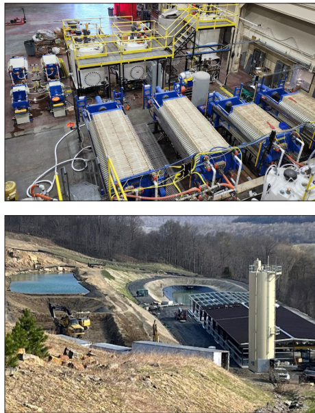
Figure 2. Small pilot facilities for processing rare earth elements from coal-based resources. Clockwise from top left lead performer and feedstock (University of North Dakota, lignite; Winner Water Services, coal ash; University of Kentucky, coal refuse and lignite; West Virginia University, acid mine drainage
