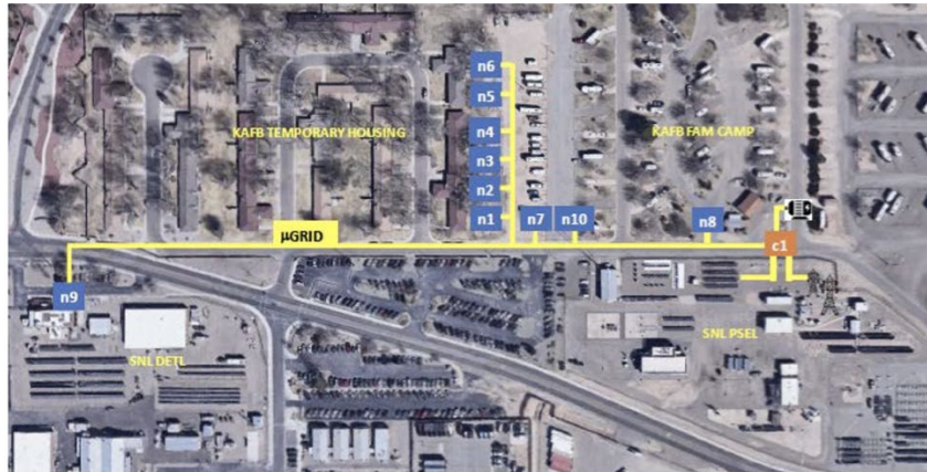
Figure 6 - Installed and operational DC/AC hybrid microgrid on Kirtland AFB. This Sandia/Emera project has been operational since December 2019
