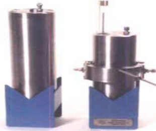
Lab-based Pressure Vessel (on loan from Schlumberger)
